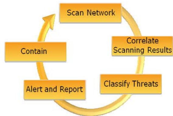
Figure 1: AirWave RAPIDS Rogue Detection automatically detects and locates unauthorized access points and utilizes a set of rules to highlight the most important threats to your organization.
